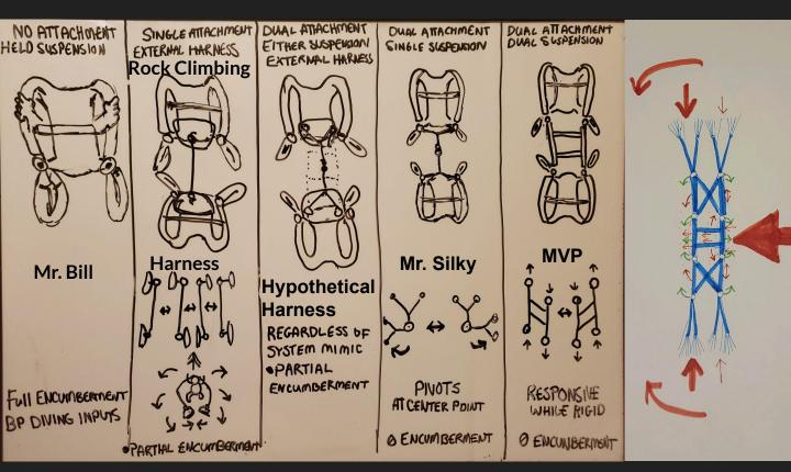
Any design with more than 2 attachment points adds unnecessary complexity. External harnesses may shift under dynamic forces and cause a loss of control. There's nothing stopping single point suspension from slamming together like a bear trap upon receiving a dock. Removing all weight and fatigue from the canopy pilots should be a top priority when building and flying any harness.
